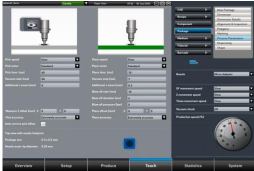
Specific settings in ePlace for accurate placement
