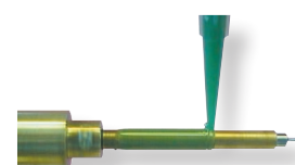
Grease dispensing on drill bits for machining
