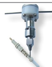
Dispensing of two-component epoxy on optical fiber connector
