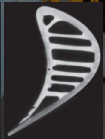
Advanced Scatter|correct cone beam CT
