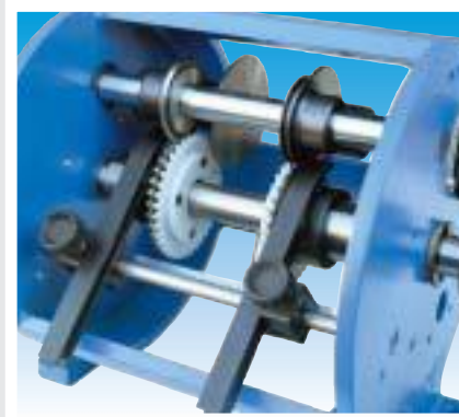
20.OL11 standard TP6 with delrin toothed discs 20.OL12 reinforced - to prevent marking the leads 20.OL11 TP6 standard con tamburi dentati in delrin 20.OL12 rinforzata - per non segnare i reofori
