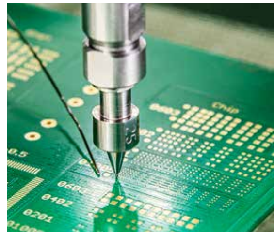
Automatic pick-up of a 01005 chip
