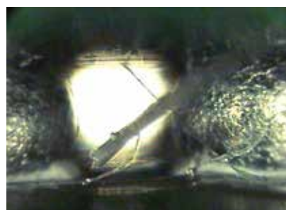
BGA: contamination (fibre)
