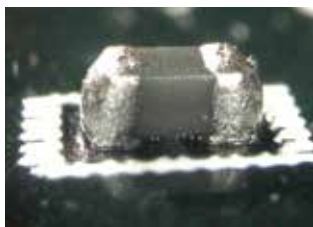
0402: bulbous solder joint
