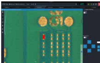
Automatically determined overlay of a 01005 chip
