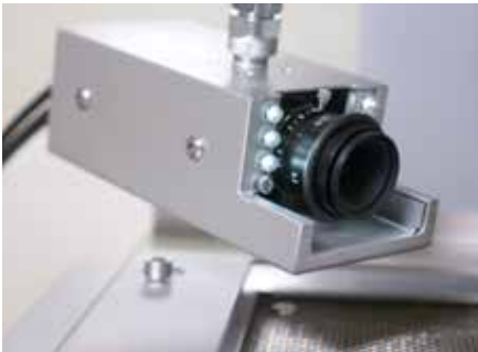
Reflow Process Camera (RPC) on the HR 550
