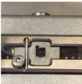
Provision of 01005 components with a tape feeder
