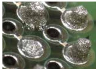
BGA - paste print: insufficient solder
