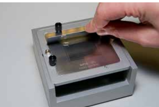
Flux deposition in the dip stencil
