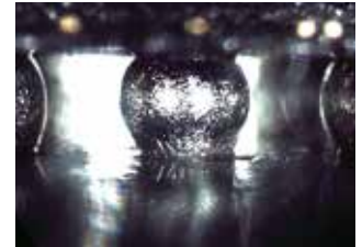
PBGA - cold joint: insufficient heat
