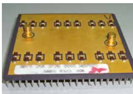
High-mass ceramic Pin Grid Array
