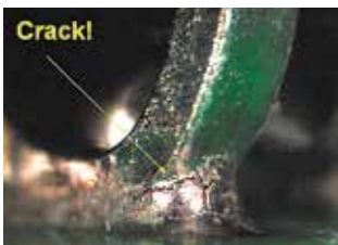
Lead-free PLCC: micro crack
