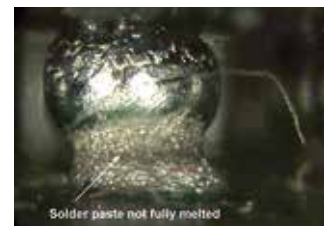
PBGA - scaling: insufficient heat
