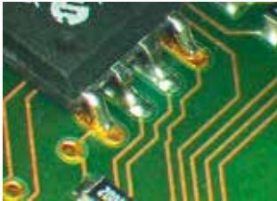
Lead-free assembly: non-wetting
