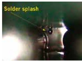
BGA: via hole solder splash
