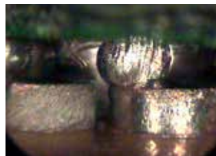
BGA - piggy back: bad alignment
