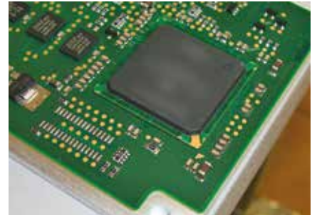
PBGA on aluminium carrier
