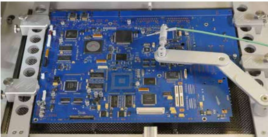
Processing an assembly in the HR 550
